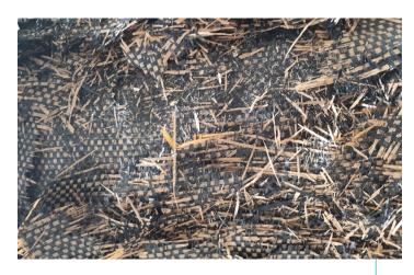
Degraded Duracover after greenhouse test
