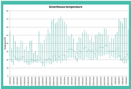
Duracover was installed in a small greenhouse facility in Lokeren, Belgium. Between the 4th of June and the 7th of August 2018, the temperature of the roll was closely monitored (see graph). Temperatures up to 72°C were registered.
